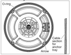
NOTICE Use a screwdriver to avoid stripping the drum cover plastic. Stop tightening when resistance is felt.
