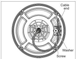
6. The end of the cable has a lot of potential energy. Be careful when removing the cable. Use your free hand to hold the cable down while the screw and washer are removed. Then, slowly remove the cable end from the anchor.
