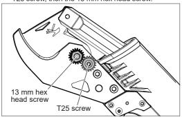
4. Remove the T25 locking cap screw.
