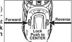
For **reverse** (counterclockwise) rotation, push in the control switch from the left side of the tool. **Check direction of rotation before use.**
