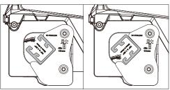
Release the return arm back into place ensuring die retaining pin is properly seated into the die.
