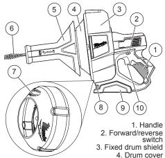
Front handle/Slide action cable lock Cable
