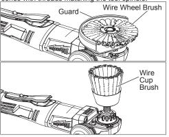
Test wheel for balance and loose or damaged wires by letting it spin for one minute before applying it to the workpiece. During this time, no one should stand in front of or in line with it.
