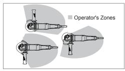
**1** To reduce the risk of injury, always use a side handle when using this tool. Hold securely.
