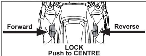
For **forward** (clockwise) rotation, push in the control switch from the right side of the tool. **Check the direction of rotation before use.**
