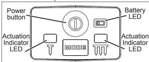
3. Press and hold the MODE button to toggle between single sequential actuation mode and contact (bump) actuation mode.
