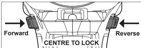
1. For **forward** (clockwise) rotation, push the control switch in the direction shown. **Check the direction of rotation before use.**
